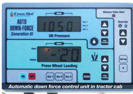
Each opener is hydraulically controlled
